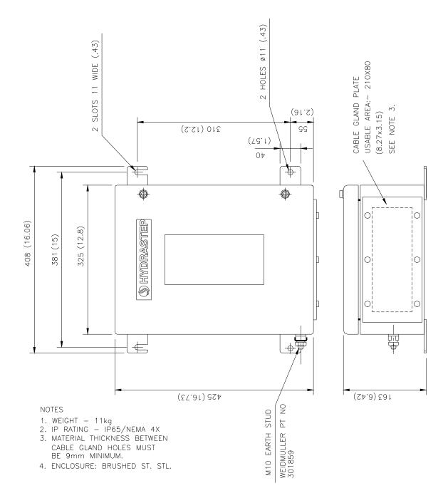
Figure 2.2: Installation diagram for Hydrastep 2468 Electronic Gauging System unit
